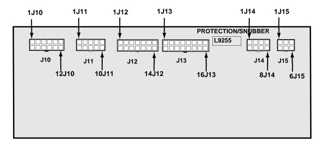
FIGURE F.6 - PROTECTION/SNUBBER BOARD TEST POINTS.
